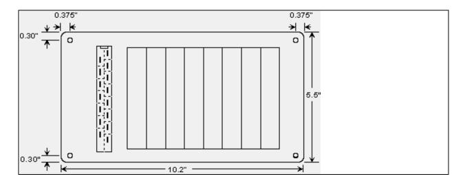
The diagram below shows the location of the four mounting holes used when mounting the unit with screws. The mounting holes are 0.188" in diameter.
