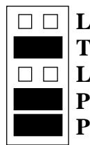
Figure 10: Headers E1 and E4= 422 with BIAS , Line Termination
