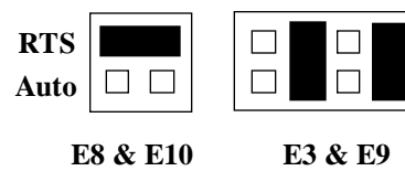
Figure 9: RS-485 'RTS' Enabled, with 'No Echo'
