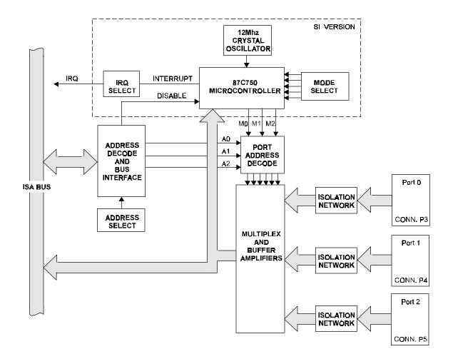
Figure 1: DIO48I Block Diagram
